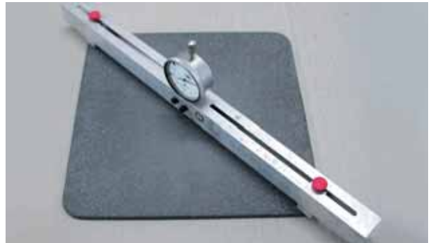
Proximity measurement of flatness at planar components
