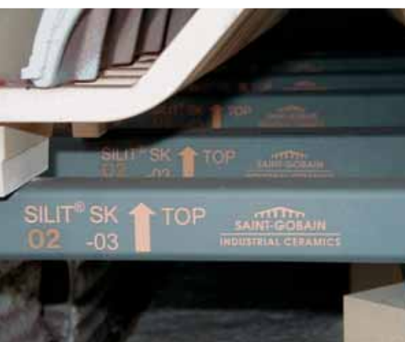
Beams out of Silit® SK and AnnaSicon® RT for firing roof tiles
